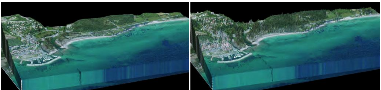
Figure 11. Examples of Digital Terrain Model (left) and Digital Elevation Model (right) (from Balouin, et al., 2013).
