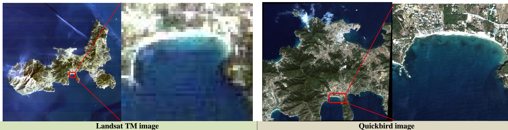
Figure 5. Elba Island (Italy) observed from multispectral imagery with a real color composition through the three spectral bands: red, green and blue (RGB). The original image and the magnified section of the same beach illustrate significant difference in the level of detail according to the spatial resolution of the satellite.
